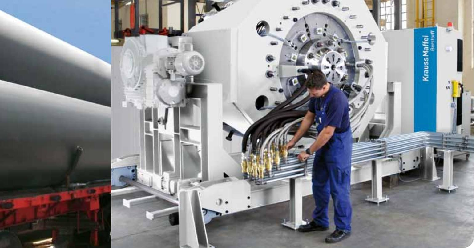
KM-RKW 39-1600 extra-large pipehead on a mounting carriage (moved aside hydraulically)
