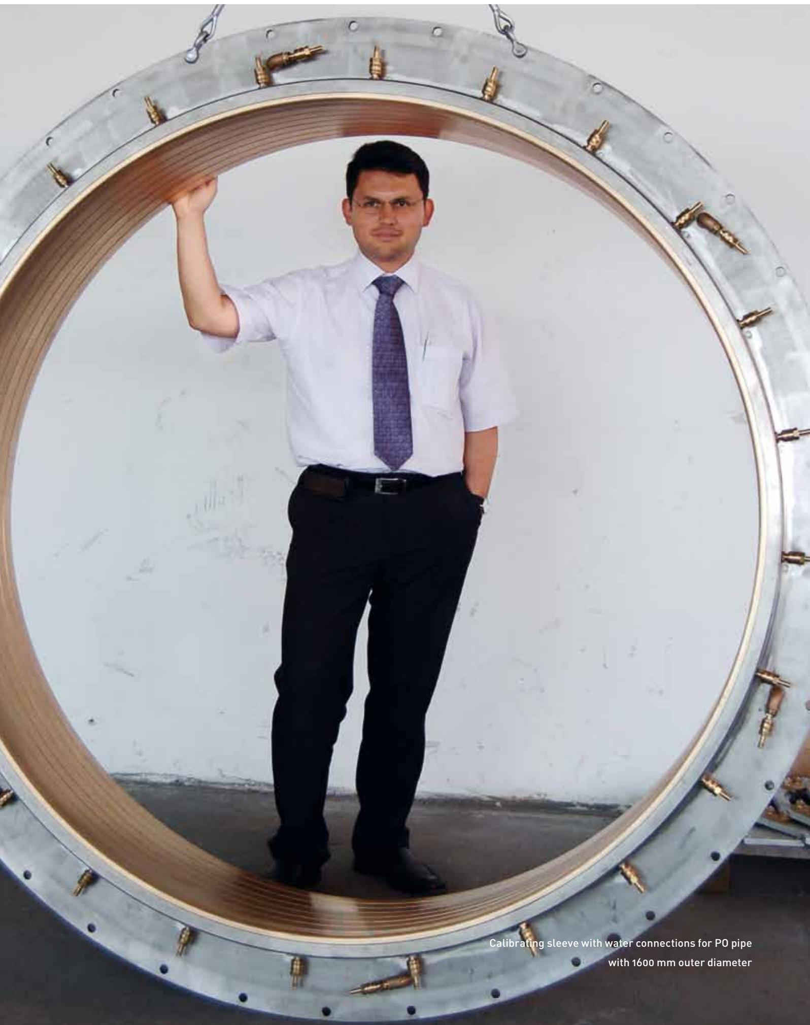
Calibrating sleeve with water connections for PO pipe
