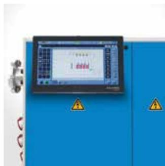
Mounted on switching cabinet door, tilting (option)
