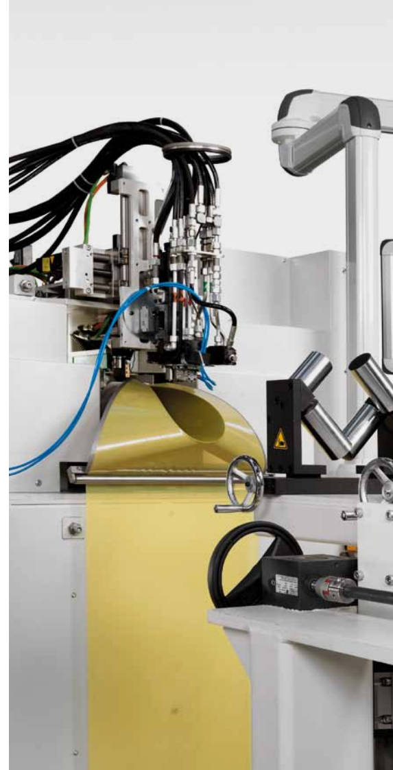
Part view: Foam-contouring unit with pipe centering station and film feed
