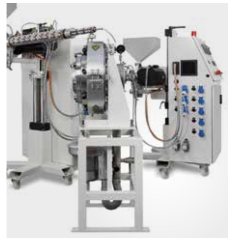
Sheathing tool KM 2L-RKW with coextruders for post-coextrusion of hot water pipes with bonding agent and oxygen barrier layer
