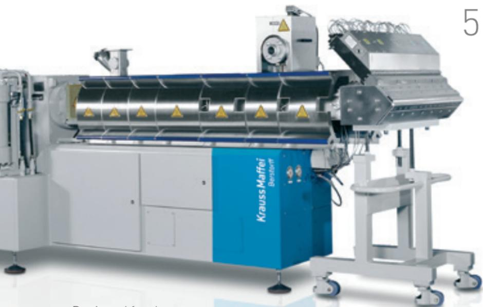
Designed for the production of EVA sheet, equipped with vacuum degassing, gear pump and special slot die featuring automatic die gap adjustment
